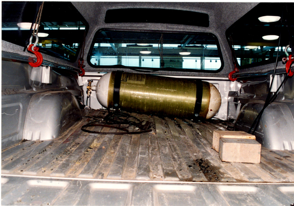
11. Add-on steel CNG tank mounted to bed of cargo box
